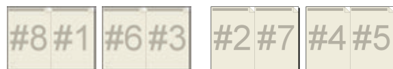
8-page saddle stitching. First sheet front and back, second sheet front and back
